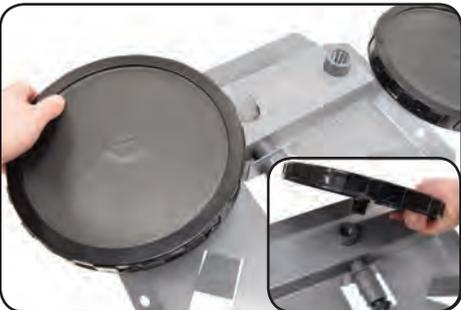
3. Screw diffuser(s) onto  $\frac{3}{4}$ " FPT on top of unit. Snug fitting by hand. Do not over tighten.
