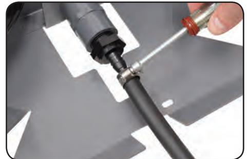
5. Slide hose clamp over fitting and fasten with regular screwdriver or nut driver.
